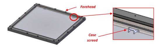
The front face is identified by the presence of one or two white polyamide slide(s) at the top of the slope.
